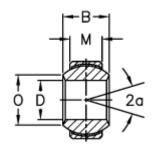
Α = 42 a (degrees) = 15 В = 28 D = 22 Dynamic load C (kN) = 97= 20 M
